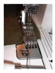
6. Cut the needle threads near the Allen wrench (Allen Key). This isn't how I cut the thread put you get the point ©
