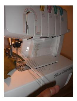
5. Lift the presser foot. Using the Allen wrench (Allen Key) that came with the machine, swipe the Allen wrench under the presser foot, from the **BACK TO THE FRONT**. This pulls the needle threads underneath the presser foot.
