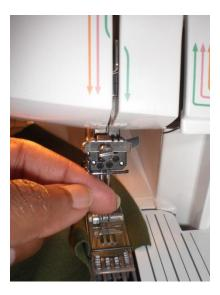
3. With your other hand push the tension lever for the same needle thread and pull the thread forward for several inches.
